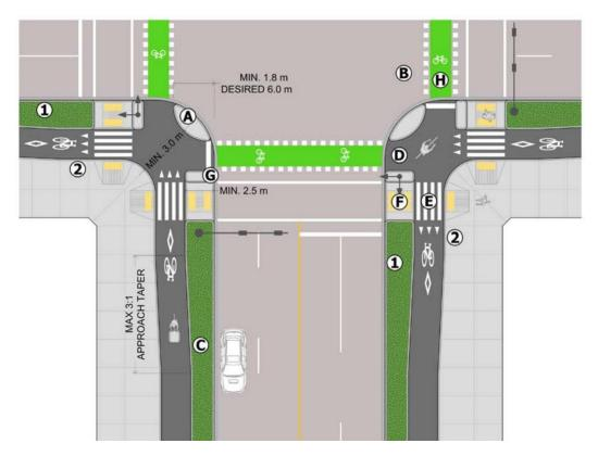
Protected Intersection with Uni-directional Protected Bike Facilities. Source: Chapter G of the BC Active Transportation Design Guide.
