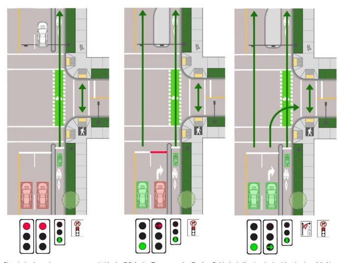
Signal phasing schemes recommended in the BC Active Transportation Design Guide including 'exclusive bicycle phase' (left), 'concurrent protected bicycle phase' (middle), and 'leading bicycle interval' (right).
