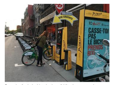
Example of a docked (station based) bike share system in Montreal, Quebec. Users can access a bicycle at a physical docking station by unlocking the bike using a membership card, cell phone, credit card or other payment methods. Docking stations are distributed through a network within a designated service area. A bicycle trip both starts and ends at a docking station.
