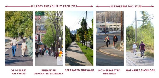
Pedestrian Facility Spectrum. Source: BC Active Transportation Design Guide, Chapter C.
