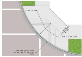
Example of a combined curb ramp. They allow people using wheelchairs to enter the crosswalk along a straight trajectory, unlike a single curb ramp that is located at an angle to the road.
