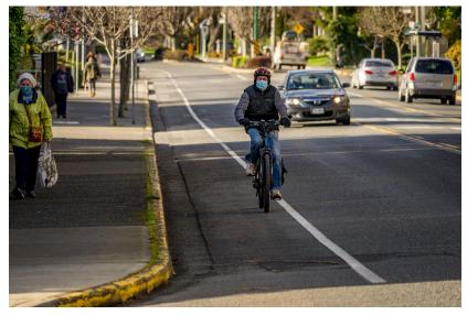
Even though a bicycle lane is provided on Esquimalt Road, with over 11,000 vehicles per day for most segments of the corridor, a protected bike facility is more suitable to meet the needs of all ages and abilities.
