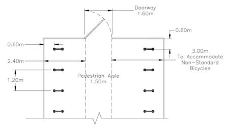
The recommended design from the BC Active Transportation Design Guide for a bicycle parking room intended for long-term bike parking.
