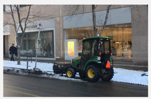
Example of a John Deere tractor from the City of Calgary that is clearing snow in a protected bike lane. This tractor has different attachments (brush, bucket, sprayer on the back) that can be used to clear snow, leaves, and other debris.
