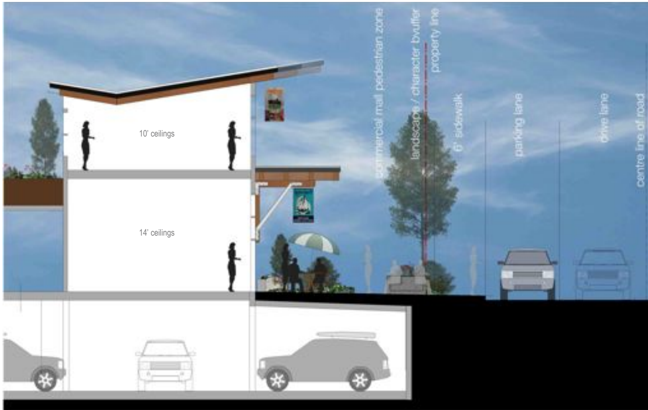
Section through Head Street Commercial Building demonstrating the value of the setbacks proposed.
