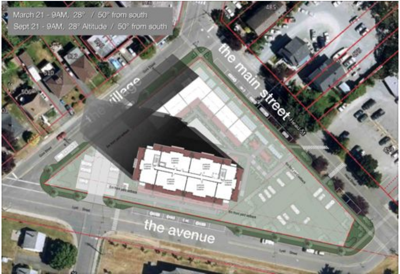
Morning shadows studies at 9AM March 21st, and September 21st, demonstrating shadows cast from both the fifth and sixth floor levels. These shadows approach but do not impose on residential properties.
