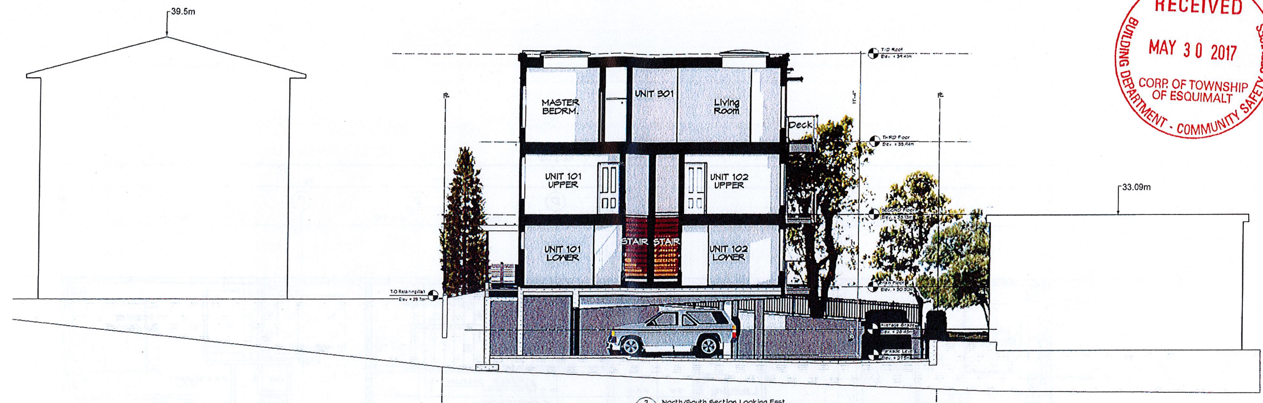
2 North/South Section Looking East Scale: 3/16" = 1'-0"
