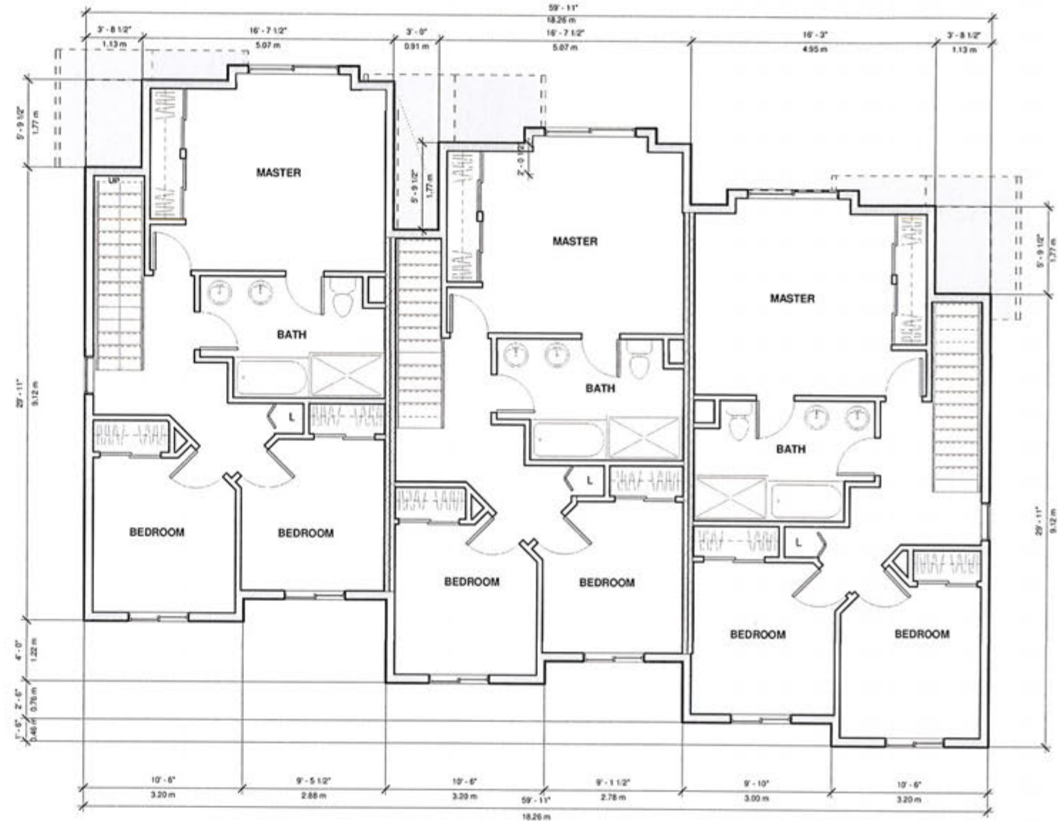
UPPER FLOOR PLAN 2041.26 SF (189.63 ms) F.A.R. 1931.29 SF (129.41 ms)
