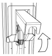
Pull out the connector and unroll the cable to an appropriate length. WARNING: Do not let the cable drag on the ground.
