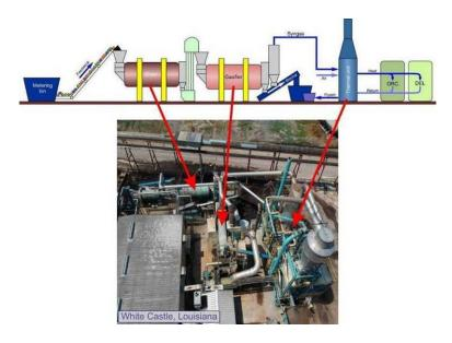
Figure 48: Schematic Overlay of White Castle Plant
