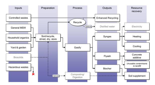
Figure 28: Gasification General Process
