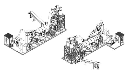
Figure 49: Gasifier Schematic
