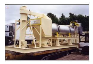
Figure 38: Mobile RotoGasifier Unit
