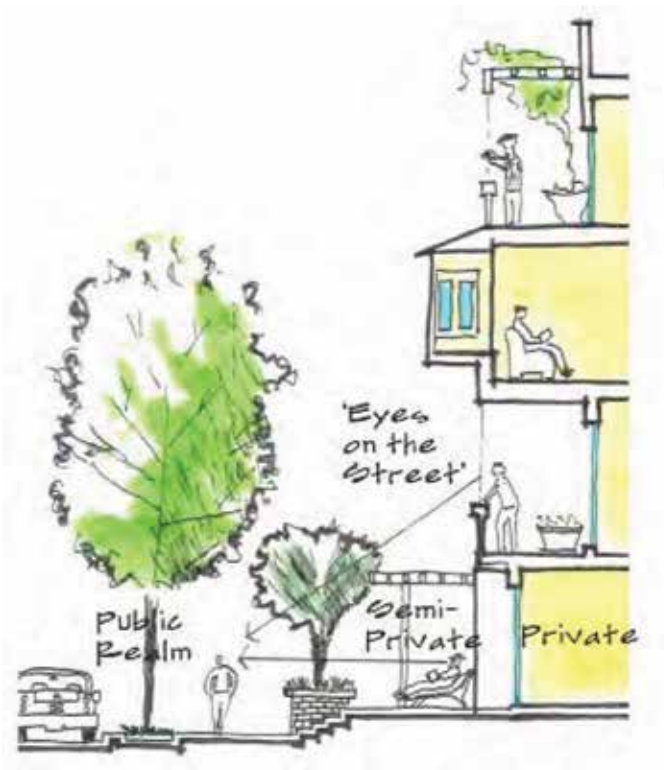
Incorporate a front patio or stoop to create street activity and association among neighbours.
