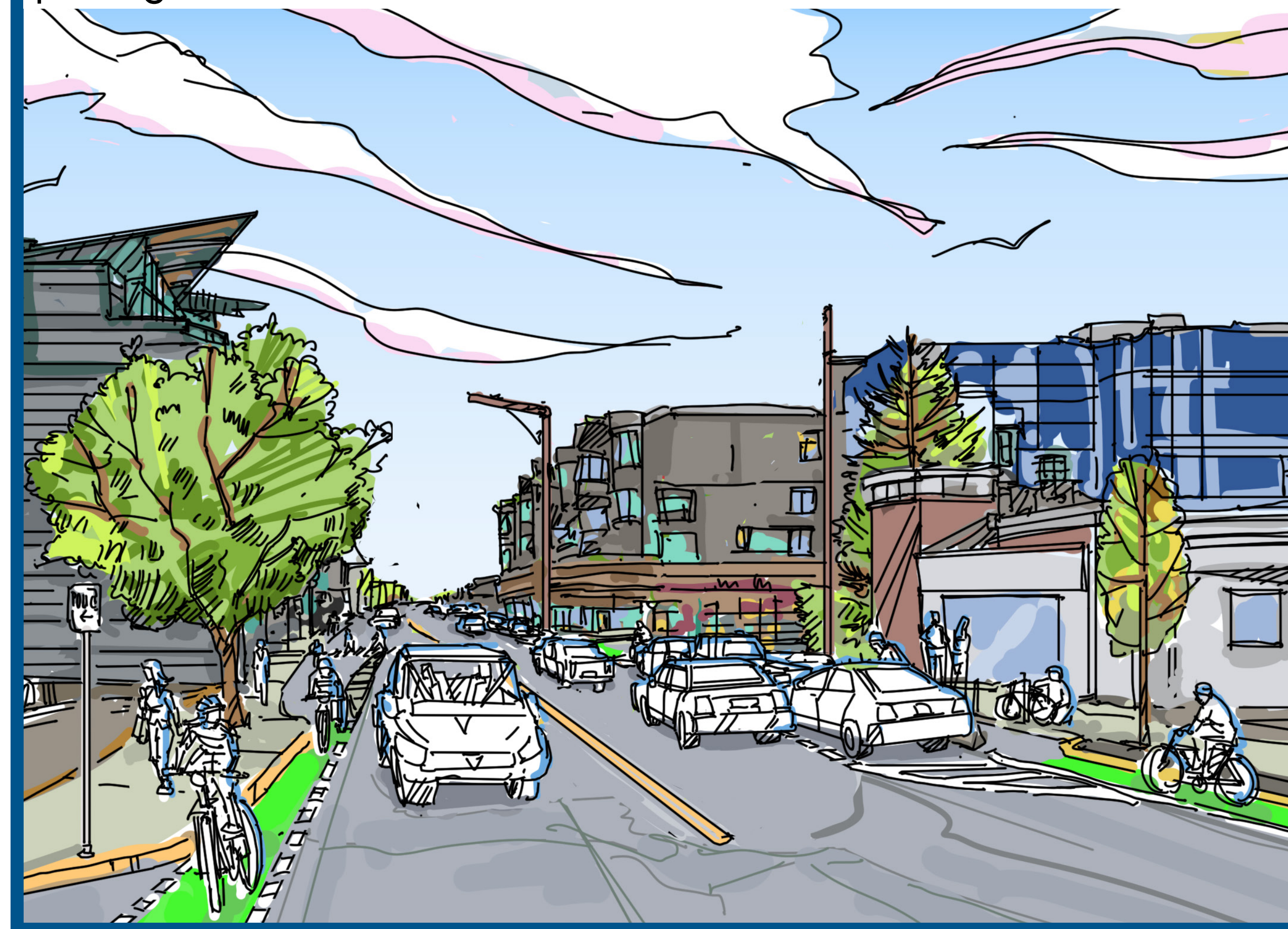
Protected bike lanes with median and turn lane removal for partial parking retention
